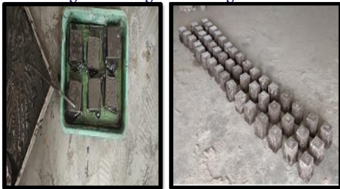
Fig. 2: Casting and Curing Process
