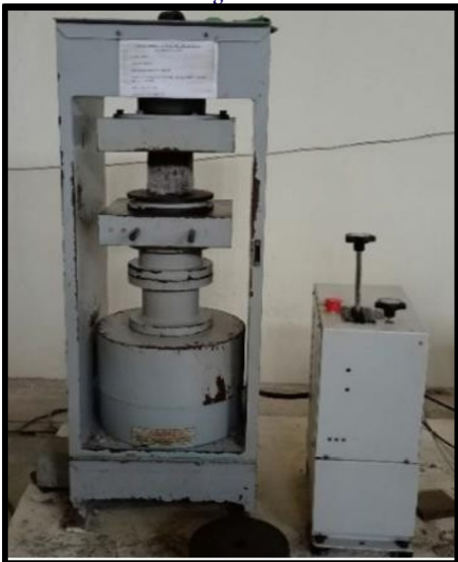
Fig. 3: Testing of Specimen in Compression Testing Machine
