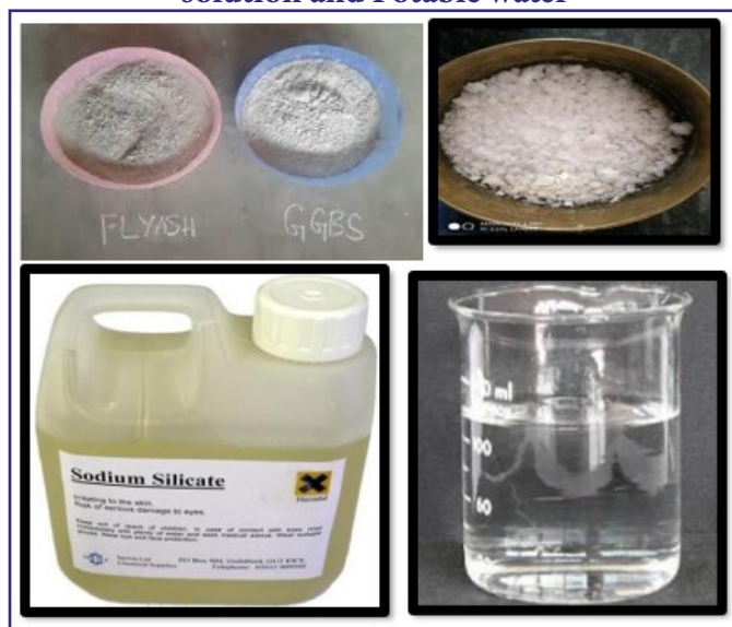
Fig. 1: Materials- Fly ash, NaOH pellets, Na 2 SiO 3 solution and Potable water
