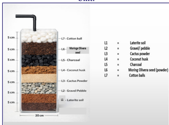
Fig. 1: Schematic Representation of Filtration Unit.
