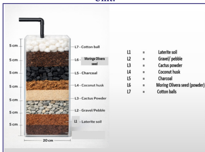
Fig. 1: Schematic Representation of Filtration Unit.
