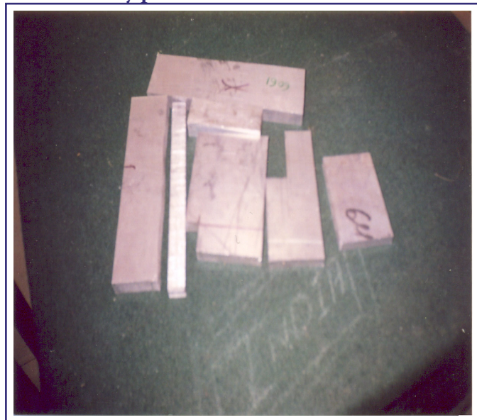
Fig. 1: provided below depicts the aluminum 6061 alloy pieces used in the research.
