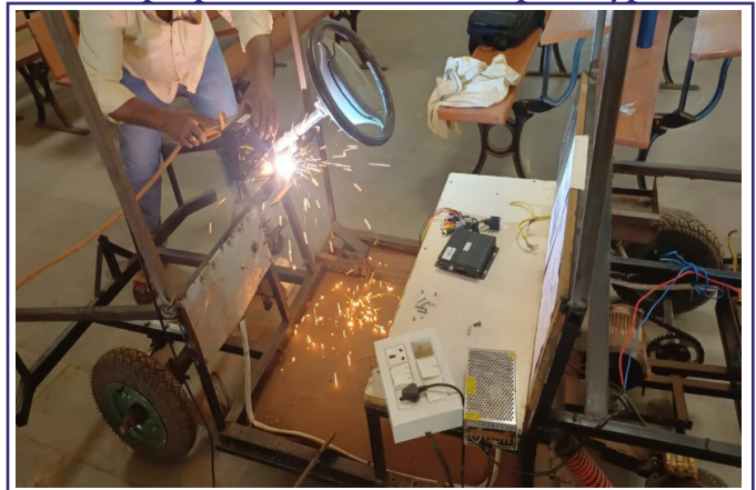
Fig. 2. Chassis fabrication and welding process of the proposed electric vehicle prototype.
