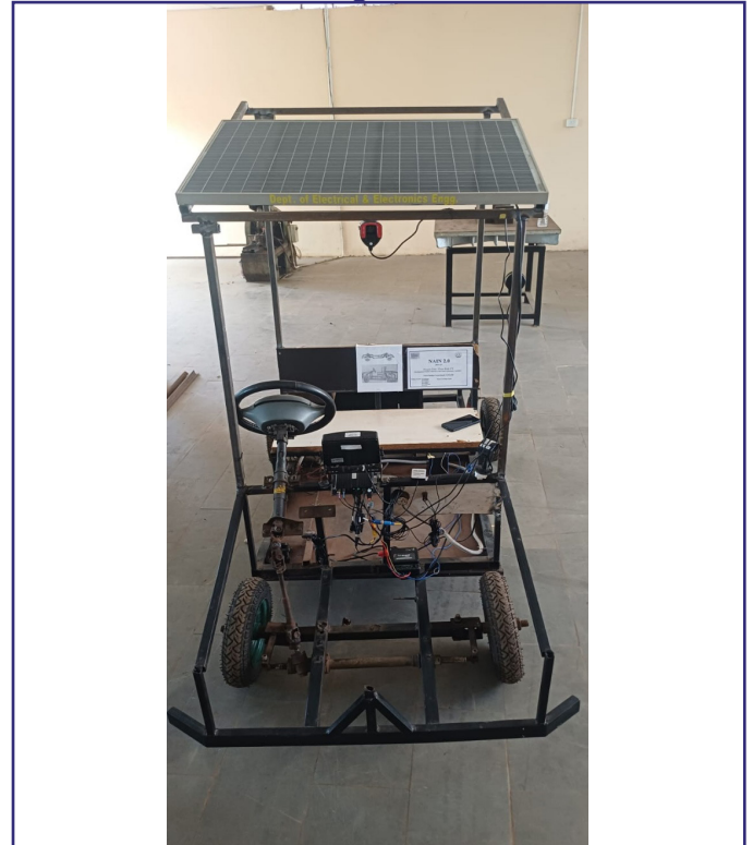
Fig. 4: Final developed prototype with solar panel integration
