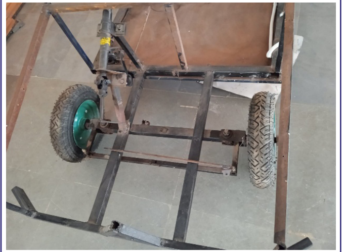
Fig. 1: Chassis fabrication and frame development
